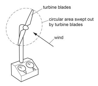
The mass of air passing through the circular area swept out by the turbine blades each second is 7.5 kg.
