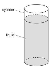
The depth of the liquid is  $10\,\mathrm{cm}$  and the radius of the cylinder is  $3.0\,\mathrm{cm}$ . The weight of the liquid in the cylinder is  $2.5\,\mathrm{N}$ .
