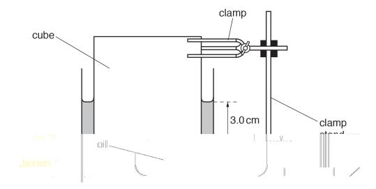
The lower face of the cube is 3.0 cm below the surface of the oil.
