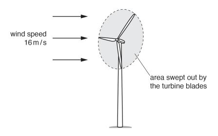
The wind blows at a speed of  $16\,\text{m/s}$  towards the turbine blades. In one second, a volume of  $24\,000\,\text{m}^3$  of air passes through the circular area swept out by the blades. The density of air is  $1.3\,\text{kg/m}^3$ .
