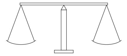
A copper block of unknown mass is placed on the left-hand pan. Six standard masses, placed on the right-hand pan, cause the balance to be in equilibrium, with the beam horizontal.
