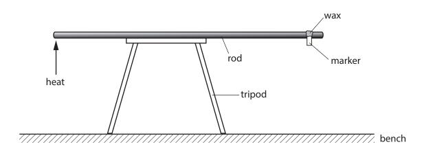
One other piece of equipment is required to compare how quickly thermal energy is conducted. Name this piece of equipment.
